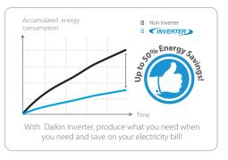
The variable speed compressor of the Inverter split continuously adjusts the power to meet the set temperature in the room; **in simple words, the unit will run at higher speed when you need more cooling and at lower speed when you need less.** The electricity you will use then depends on your actual needs, not more! Inverter technology will lower the consumption of the air conditioner up to 50%, so you pay less money for your electricity bills!
