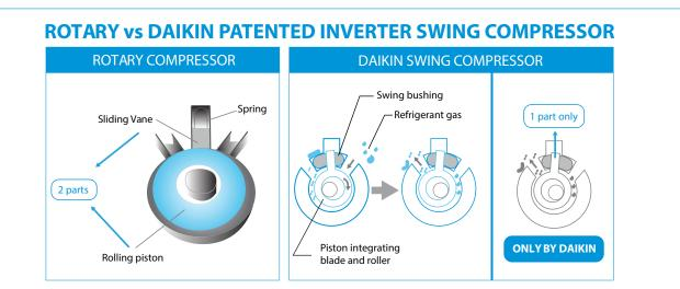
In the rotary compressor, used in traditional split air conditioner, the blade serves as a partition between the high and low pressure sides, and the gas refrigerant is compressed as the rotor rotates. The blade moves up and down along with the rotation of the rotor.
